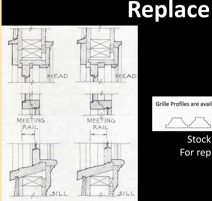
Grille Profiles are available in widths ranging from 5/8" to 2-1/4"
