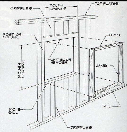
Figure 11.1 Window assembly in wood frame construction.
